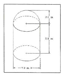
10) Determine the mass of the part shown if it is constructed from material that has a density of 0.0008 kg/cm<sup>3</sup>. Density is mass per unit volume  $\left(D = \frac{M}{V}\right)$
