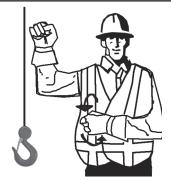
TRAVEL. (One Track). Lock the track on side indicated by raised fist. Travel oppsite track in direction indicated by circular motion of other fist, rotated vertically in front of body. (For crawler cranes only.)
