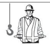
EXTEND BOOM. (Telescoping Booms). Both fists in front of body with thumbs pointing outward. One hand signal may be used.
