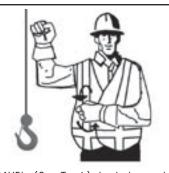
TRAVEL. (One Track). Lock the track on side indicated by raised fist. Travel opposite track in direction indicated by circular motion of other fist, rotated vertically in front of body. (For crawler cranes only.)
