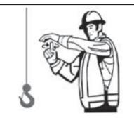
MOVE SLOWLY. Use one hand to give any motion signal and place other hand motionless in front of hand giving the motion signal. (Hoist slowly shown as example).
