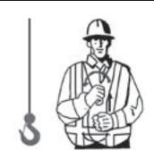
TRAVEL. (Both Tracks). Use both fists in front of body, making a circular motion about each other, indicating direction of travel; forward or backward. (For crawler cranes only.)
