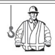
RETRACT BOOM. (Telescoping Booms). Both fists in front of body with thumbs pointing toward each other. One hand signal may be used.
