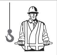
EXTEND BOOM. (Telescoping Booms). Both fists in front of body with thumbs pointing outward. One hand signal may be used.
